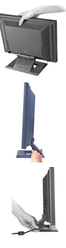
4. Connect the other end of signal cable to the signal connector of your computer.
